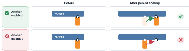
Figure 3. Effect of anchor recomputation after parent resizing. With recomputation, the child follows the updated parent anchor; without it, the child remains at its pre-edit position.
